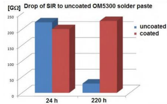
Figure 2.46: a) Assembled B52 advanced test board and SIR data with 25-55 °C, 96 %rH cyclic condition, 26-1 – 26-7 refer to different patterns on the B52 test board [115]. b) SIR values for two solderpaste-comb patterns with coating and without coating, 24 hours and 220 hours into an SIR test at 40 °C/90 %rH [125].
