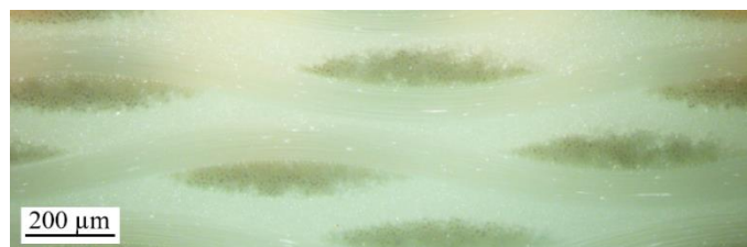
Figure 2.6: Exemplary cross section of an FR-4 laminate consisting of epoxy resin with interwoven glass fibers.
