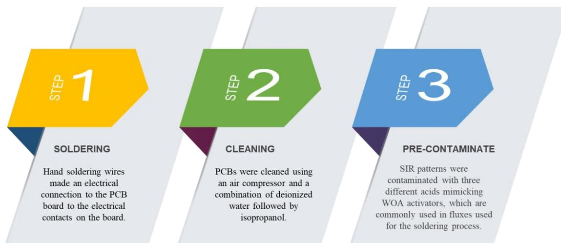
**Figure 3.2** Three Steps before DC measurement and placing the specimens inside the climatic chamber.
