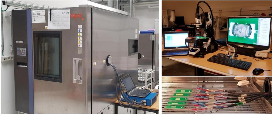
**Figure 3.3** Espec climatic chamber, BioLogic VSP potentiostat with five channels, and VHX digital microscope.
